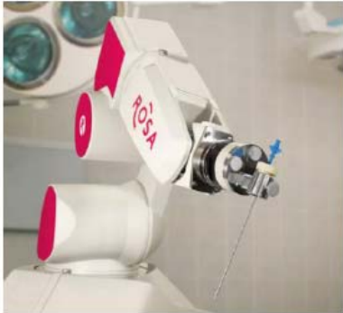
ROBOTIC ARM WITH 6 DEGREES- OF-FREEDOM
